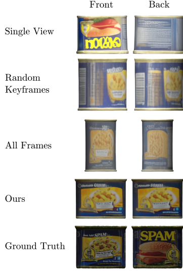
Fig. 10. Effect of keyframe selection on object reconstruction. Random keyframe selection and using all frames for reconstruction degrade the canonical reconstruction (shape/scale) compared to our balanced keyframe selection; ground truth shown for reference.
