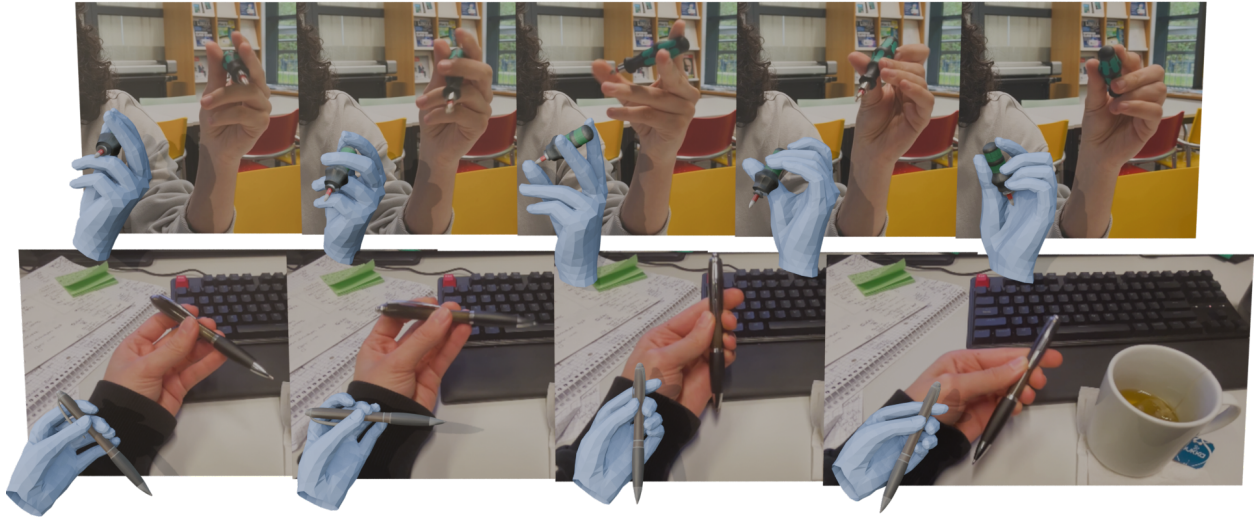
Fig. 1. Grasp in Gaussians (GraG) : Given a single monocular video of a hand interacting with an object, GraG reconstructs 3D geometry and pose of the hand and the object. Our method is designed to be efficient for long sequences, and can reconstruct in-the-wild captured examples.
